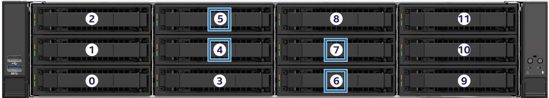
Figure 29. 2U 12 x 3.5" M50CYP2UR312 Front Drive Bay Configuration
