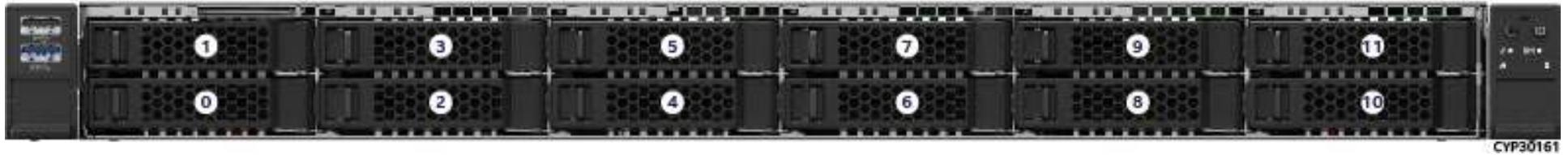
Figure 23. 12 x 2.5" Front Drive Bay Configuration – M50CYP1UR212
