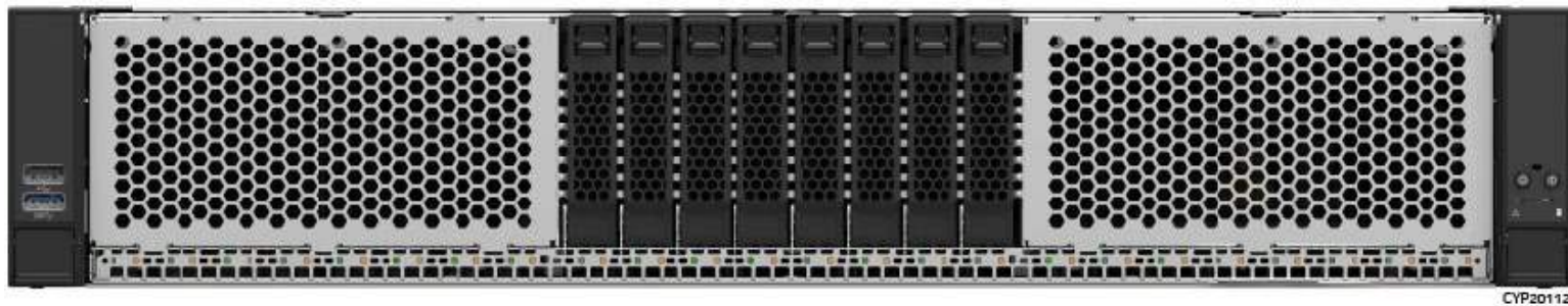
Figure 10. 2U 8 x 2.5" Front Drive Bay Configuration – M50CYP2UR208
