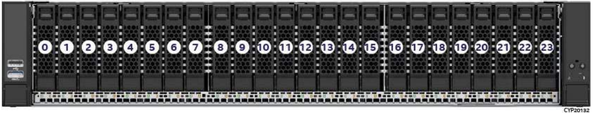
Figure 27. 2U 24 x 2.5" M50CYP2UR208 Front Drive Bay Configuration
