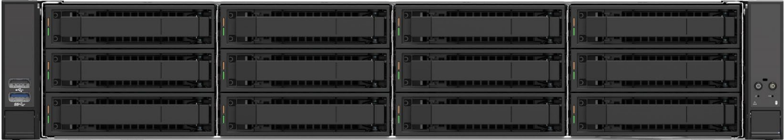
Figure 13. 2U 12 x 3.5" Front Drive Bay Configuration – M50CYP2UR312
