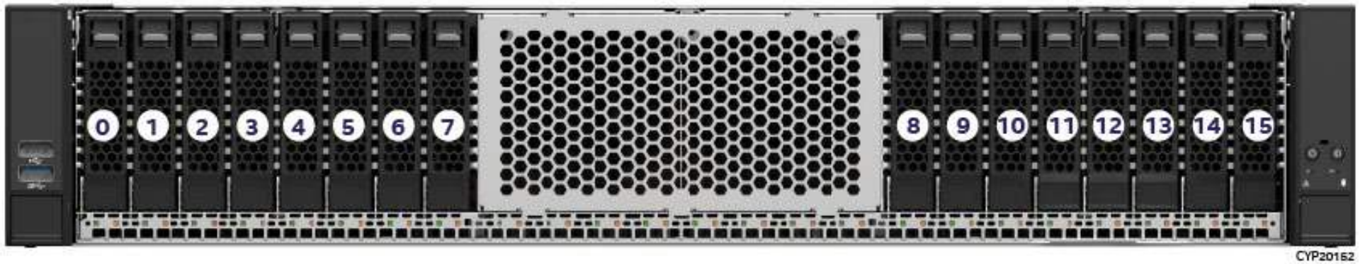
Figure 25. 2U 16 x 2.5" Front Drive Bay Configuration
