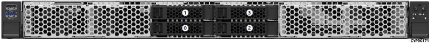
Figure 22. 4 x 2.5" Front Drive Bay Configuration – M50CYP1UR204
