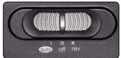
3-mode power switch: Auto / Off / Rev
